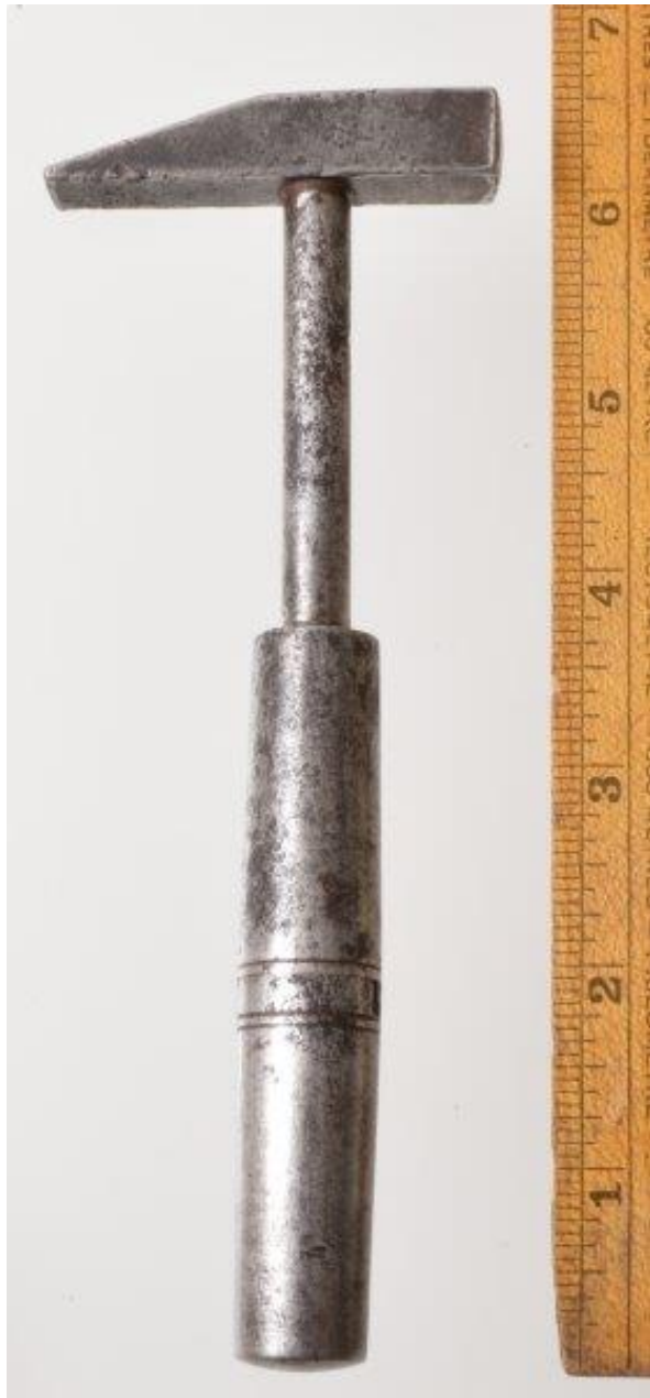
KTT024 Roundlet tool kit with hammer screwing in the end. The other tools fit in the handle slot to make a T. $19
