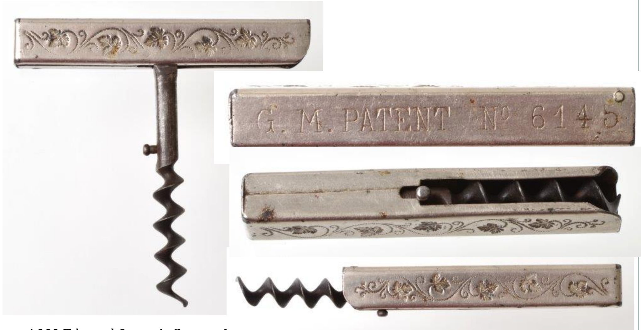
A032 Edmund Jansen's German Registered Design No. 6145 of June 27, 1892, for a corkscrew which slides out of a channel formed by folding sheet metal into a rectangle. One end and half of the underside are left open for the sliding mechanism. A backspring is located in the top of the handle and attached to it is a worm with sliding mechanism. The worm slides out the end and is turned perpendicular to the handle locking with the backspring. Marked G. M. PATENT NO. 6145. $69
