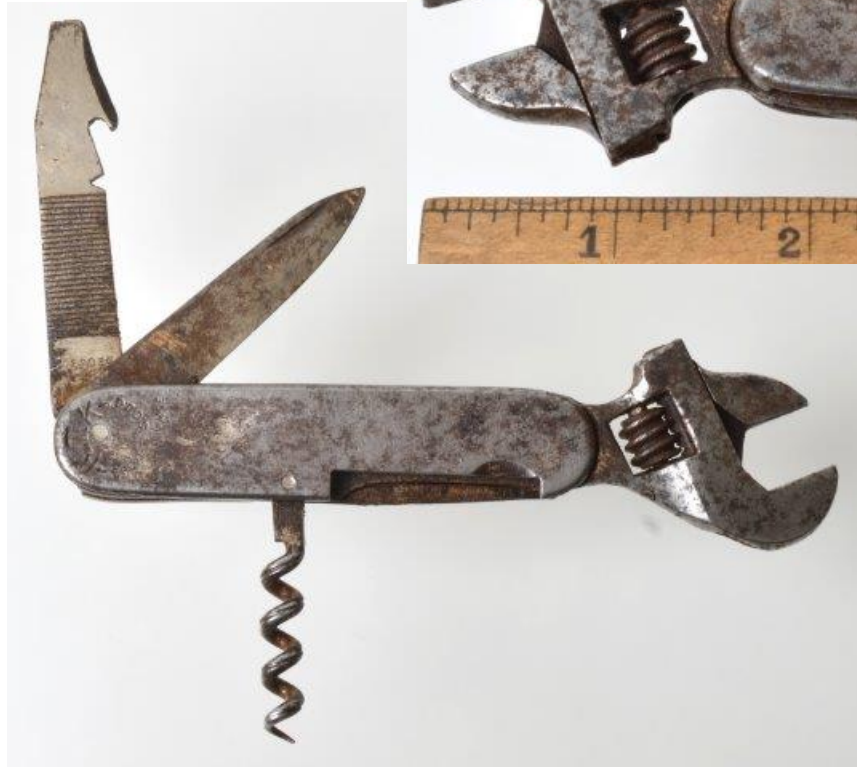
FR131 Crescent wrench with corkscrew and additional tools. On June 27, 1928, Jean-Albert Soustre was granted French Patent Number 645,624 for his " couteau à usages multiples avec clé a molette ." On June 30, 1931, he obtained an American patent (No. 1,811,982) for his tool entitled "Knife adapted for multiple uses and comprising a monkey wrench." Marked K T K BREVETE S.G.D.G. Rust, pitting, dented. $39
