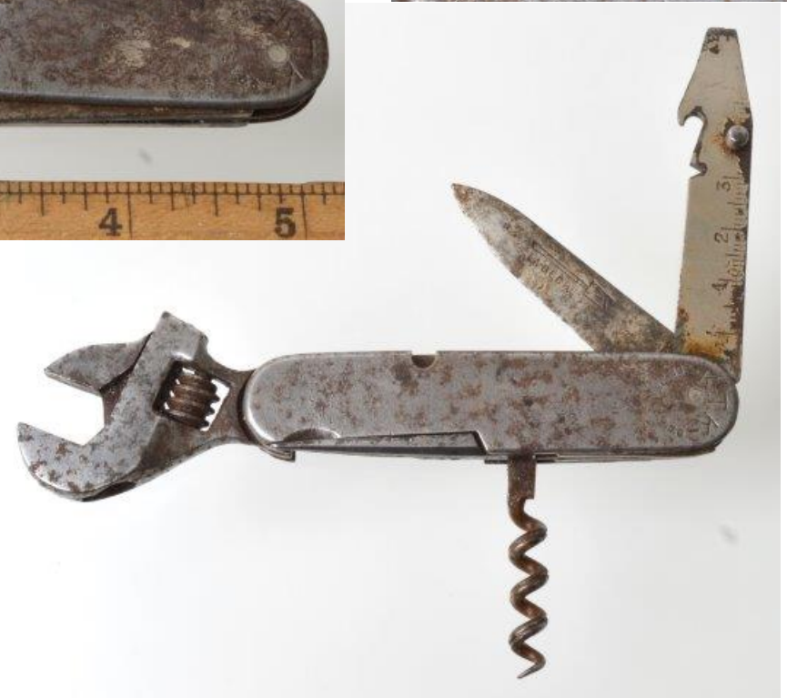
FR131 Crescent wrench with corkscrew and additional tools. On June 27, 1928, Jean-Albert Soustre was granted French Patent Number 645,624 for his " couteau à usages multiples avec clé a molette ." On June 30, 1931, he obtained an American patent (No. 1,811,982) for his tool entitled "Knife adapted for multiple uses and comprising a monkey wrench." Marked K T K BREVETE S.G.D.G. Rust, pitting, dented. $39
