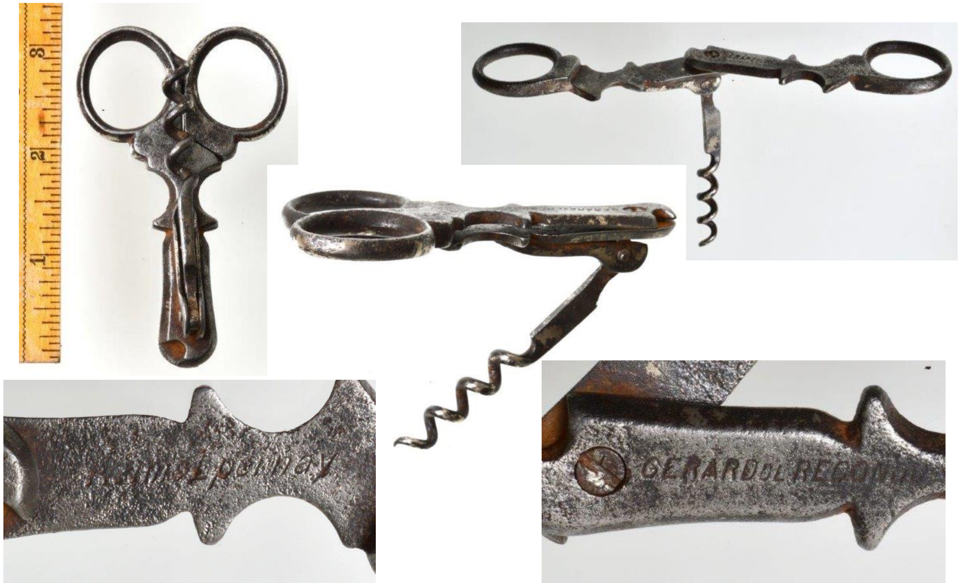
C04 Scissor style combination nipper, cigar cutter, and corkscrew. The worm unfolds from a channel which has a backspring to lock the worm in position. Advertising "Gerard De Reconde, Reims Epernay". $75
