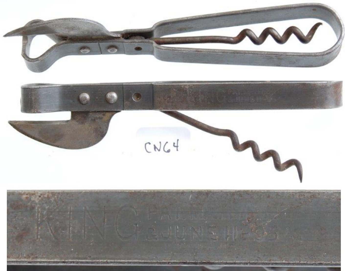
CN64 Combination tool marked KING PAT MAY 17-92 & June 11-95 with the image of a crown. U. S. Patent Numbers 475,222 and 541,034 issued to William G. Browne. $12
