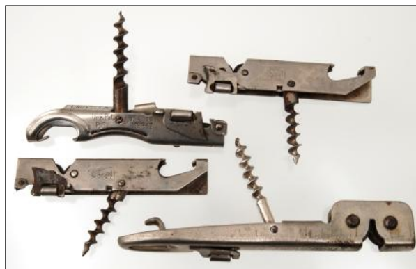
Three combination tools. Left two: One marked LAYFA INOX 18/8, other has logo only; includes sardine can opener. Right: Marked PICNIC, includes screw driver,
